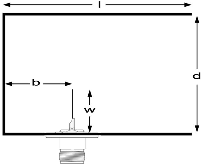
3. Mark and drill a small hole at the right position. Putting a piece of wood into the can can help stabilize it as you drill. Extend the hole step by step to the right size for the N connector to fit through.
