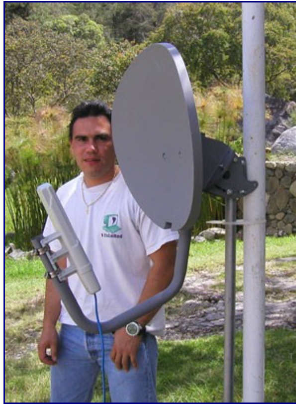
Figure 10: Motorola Canopy wireless router with parabolic reflector to increase gain
