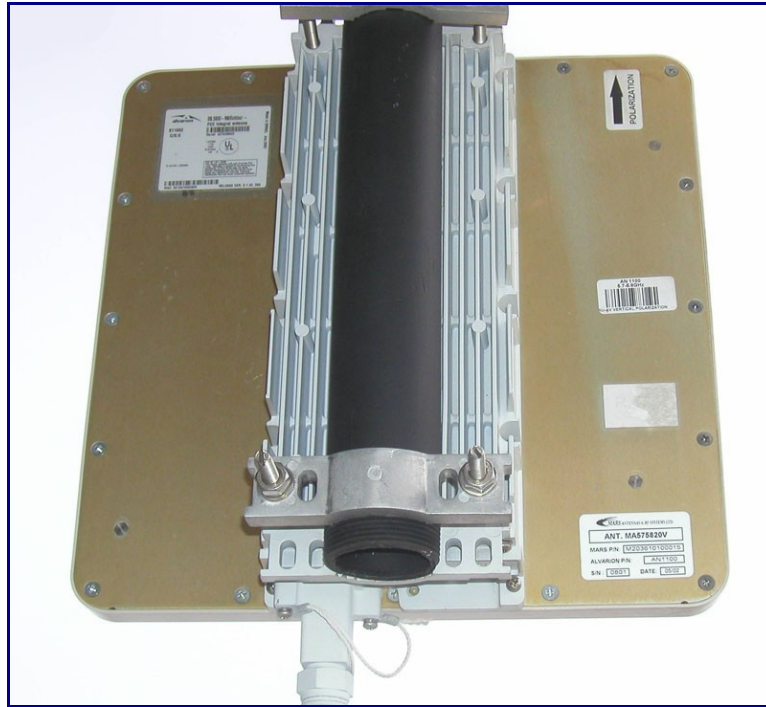
Figure 7: Alvarion DS5800 outdoor unit with patch antenna.
