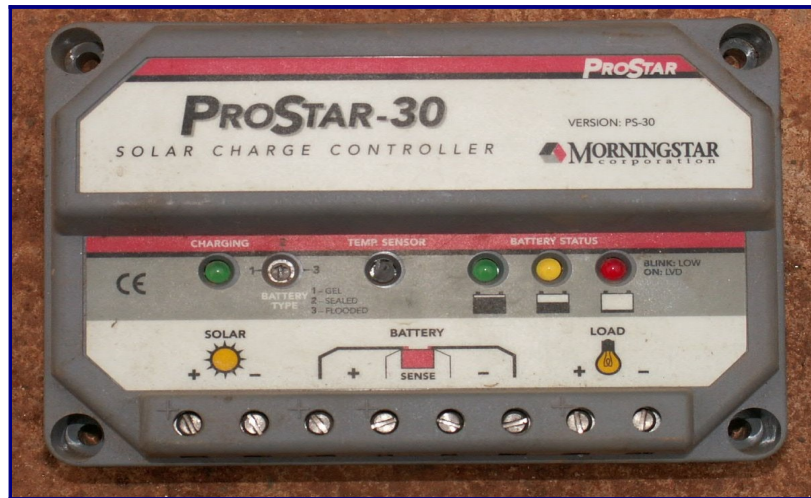
Figure 4: Solar charge controller or regulator of 30 A
