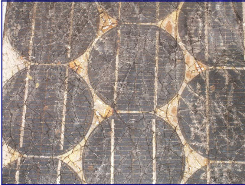
Figure 6: The effect of water and corrosion in a solar panel
